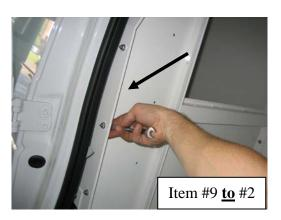
Bolt 3<sup>rd</sup> Compartment Divider to Passenger side Wall using ½" x ¾" carriage bolts, washers and nuts.
